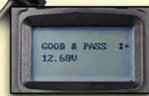
5 TEST RESULTS: A.GOOD & PASS B.GOOD & RECHARGE C.RECHARGE & RETEST D.BAD & REPLACE E.BAD CELL & REPLACE
